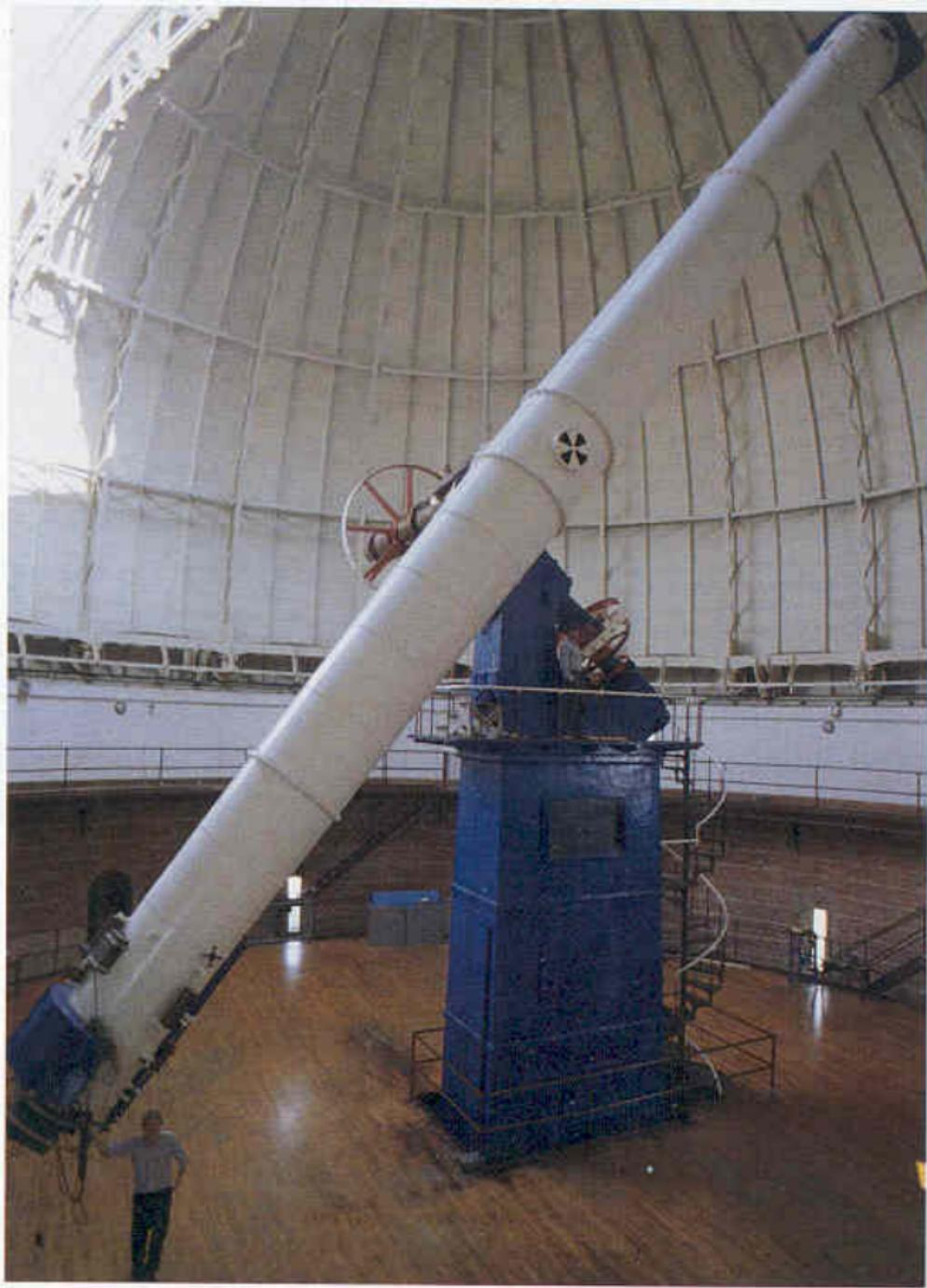
**Figure 5.6 Largest Refracting Telescope** Photograph of the Yerkes Observatory's 40-inch-diameter refractor. (Yerkes Observatory)
